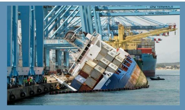
2011 the vessel was identified a Deneb a 508 TEU feeder vessel which capsized while berthed at APM Terminal's container facility at the port of Algeciras .
