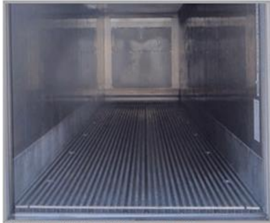
Container interior : T floor and walls
