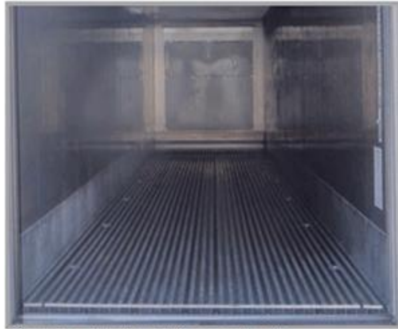
Container interior : T floor and walls
